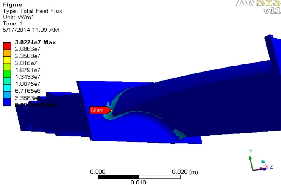
**Figure 4.1 Total heat fluxes in the blade geometry**
