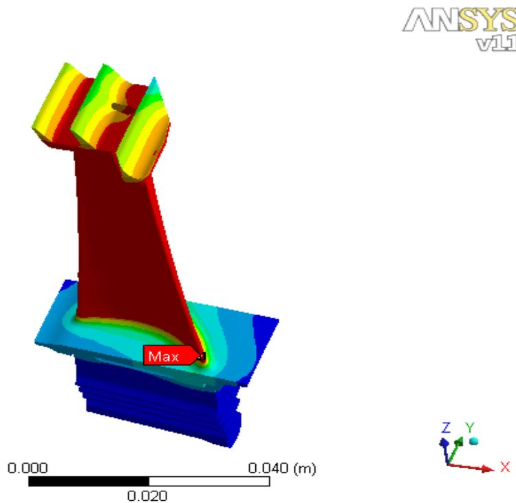
Figure 4.1 Temperature distributions in the blade geometry
