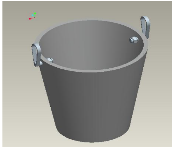
Figure 4.1 Isometric Drawing of Cylindrical-type furnace
