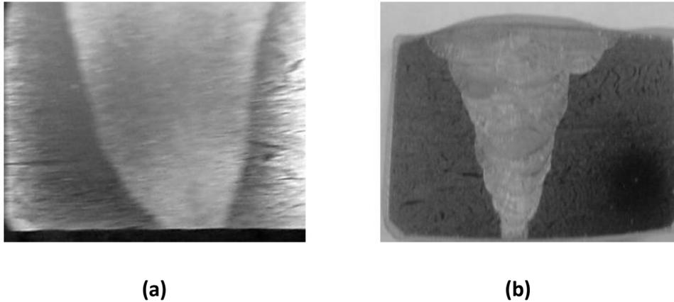
**Fig. 2 Cross-sections of the type 304LN stainless steel weld (10 mm thick) produced by (a) A-TIG welding (b) Multi-pass TIG welding**
