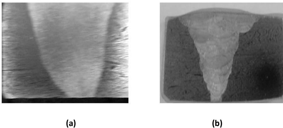
**Fig. 3 Cross sections of the type 316 LN Stainless steel weld (12 mm thick) produced by (a) A-TIG welding (b) Multi-pass TIG welding**
