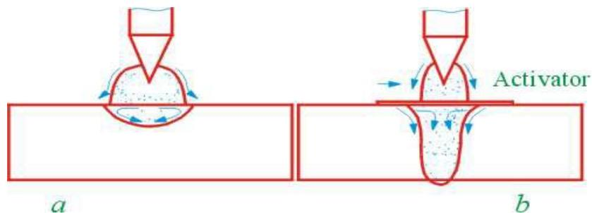
Fig. 1 Schematic sketch of (a) TIG and (b) A-TIG welding processes
