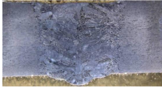
Figure 4. Cross section of ATIG welded joint; plate thickness is 8 mm.
