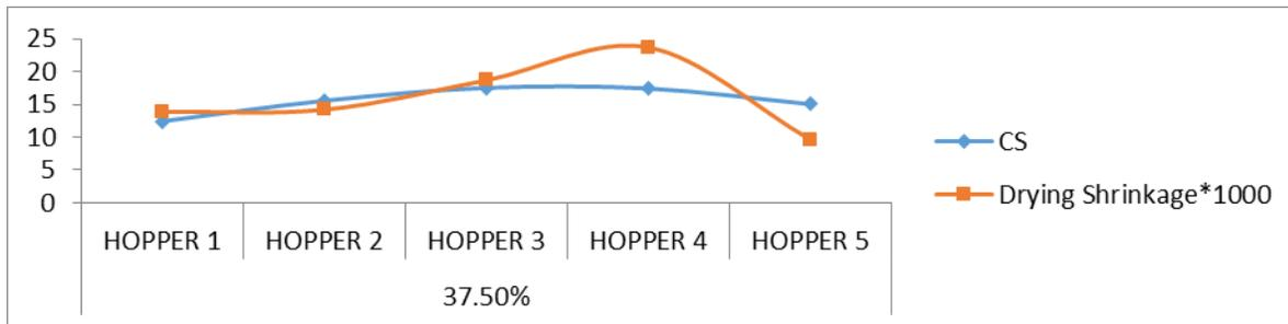
**Graph: Relation between Compressive Strength and Drying Shrinkage for varying percentage of fly ash for different fineness.**
