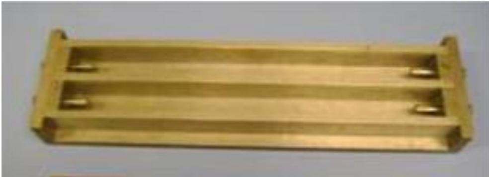
Figure: drying shrinkage mould specimen (source: google)
