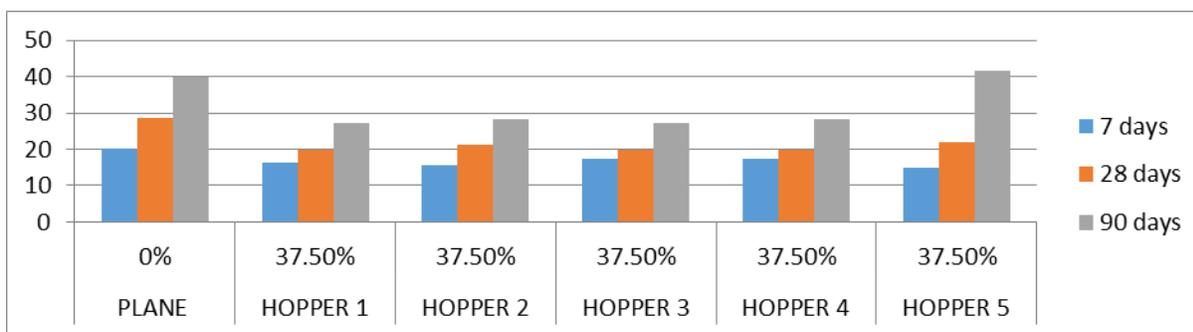
**Graph: Compressive strength result for varying percentage of fly ash for different fineness**
