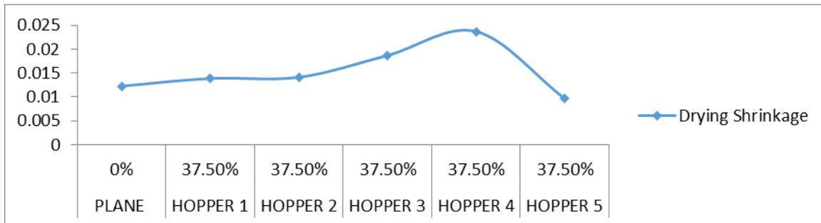
**Graph: Drying Shrinkage result for varying percentage of fly ash for different fineness.**
