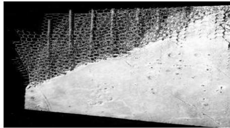
**Fig. 3 A Typical Ferrocement Section**
