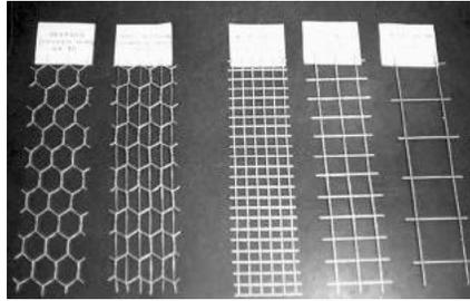
**Fig. 1 Hexagonal and Welded Wire Mesh.**
