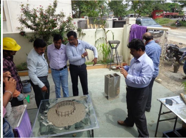
Pic 4:- Test for J ring satisfies passing ability requirements of S.C.C.
