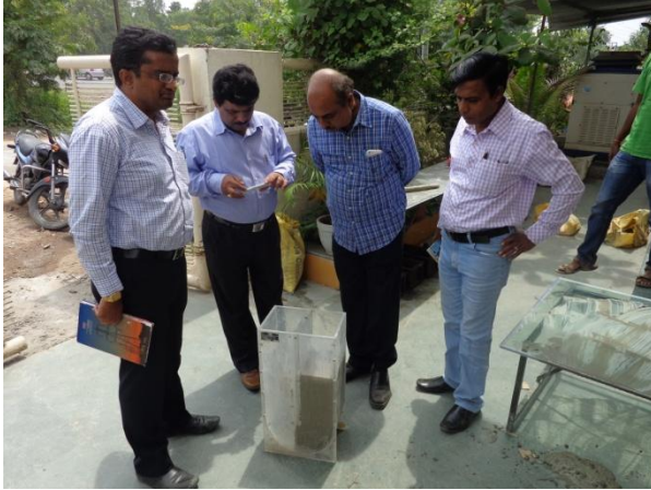
Pic 3:-Test for U box satisfies passing ability requirements of S.C.C.,
