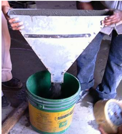
Pic 5:-Test for V funnel at T5 minutes satisfies Segregation resistance of S.C.C.
