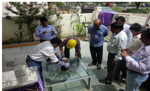
Pic 2:- Test for slump flow satisfies filling ability of S.C.C.
