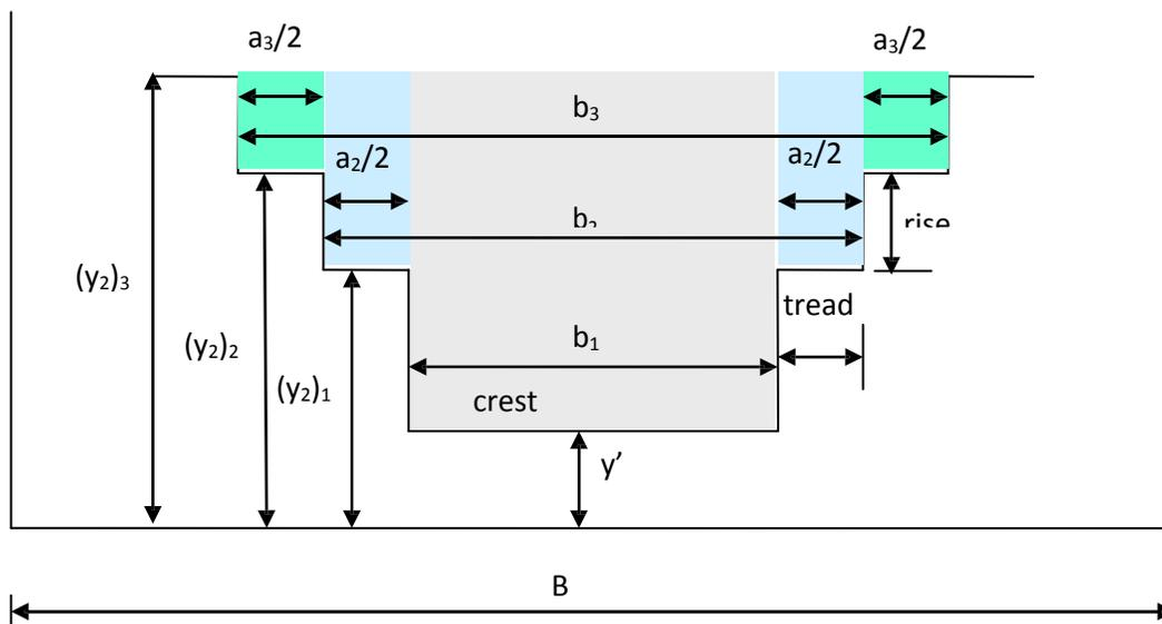
**Fig.3. Design of stepped weir (first 3-steps shown)**
