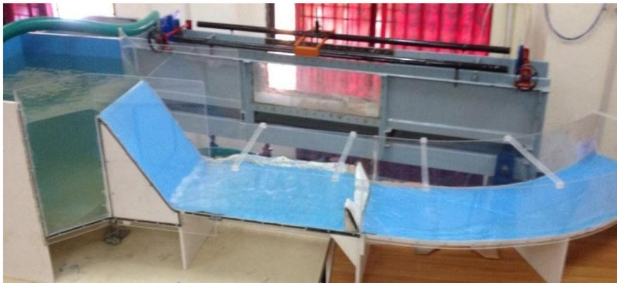
**Fig. 2. Experimental setup of Sonurle M.I. Tank spillway and energy dissipator.**
