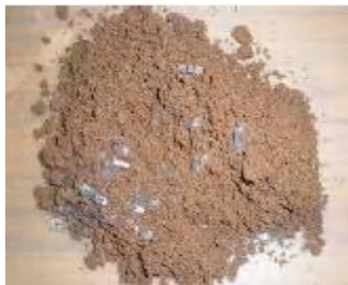
Figure 2. Plastic Waste Mixed Soil
