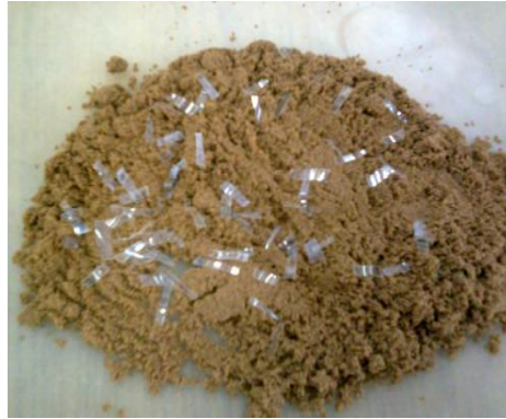
Figure 3. Sand Mixed with Plastic Waste
