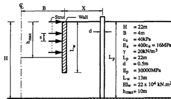
Fig 2.1: Finite Element model with strutting system
