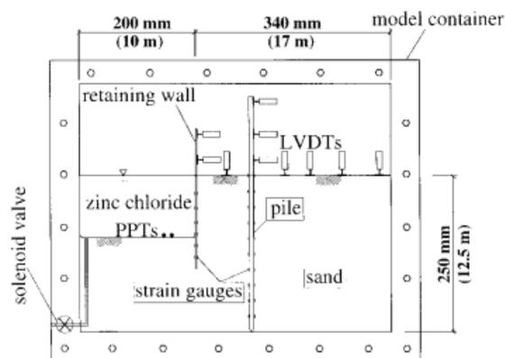
Fig 2.2: Centrifuge Model Setup for Sand
