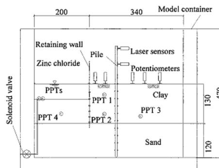
Fig 2.3: Centrifuge Model Setup for Clay
