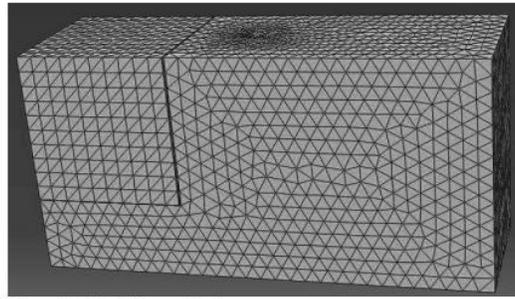
**Fig 2.4:Finite Element model of excavtion near pile in sand**
