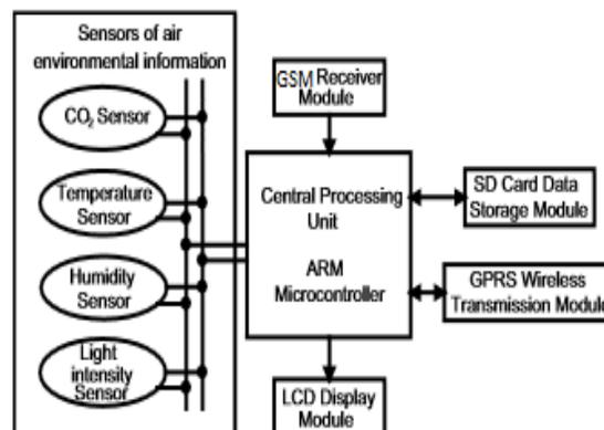
Fig 1. Hardware infrastructure diagram of geological CO<sub>2</sub> leakage monitor.
