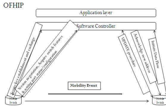
**Figure. 6: Secure Handover-update procedure**
