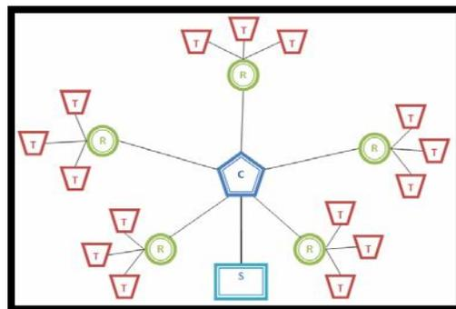
Fig 4.1: Architecture of the hybrid WSN -RFID network [13].
