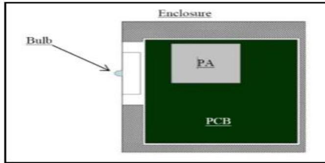
Fig.1-Lifi Block Diagram [15]
