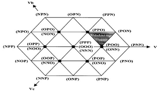
Fig-5. Space-vector diagram of the three level inverter.
