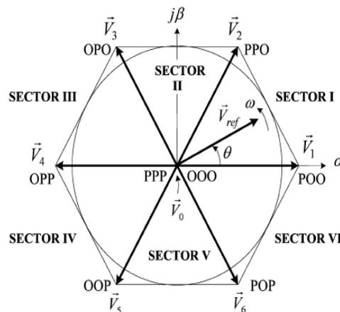
**Fig-1 Space-vector diagram - Two-level inverter.**
