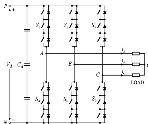
**Fig-2 Two-level Cascaded H-Bridge Inverter.**
