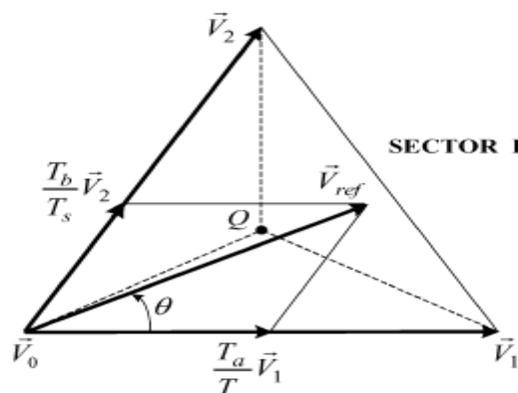
**Fig-3.  $V_{ref}$  synthesized by  $V_1$ ,  $V_2$  and  $V_0$ .**
