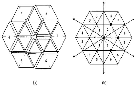
Fig-6 Simplification of a three-level space-vector diagram. Source- [6].
