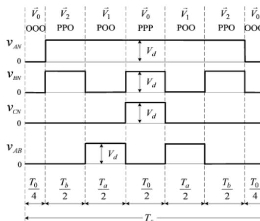
Fig-4. Seven-segment switching order for  $V_{ref}$  in sector I.
