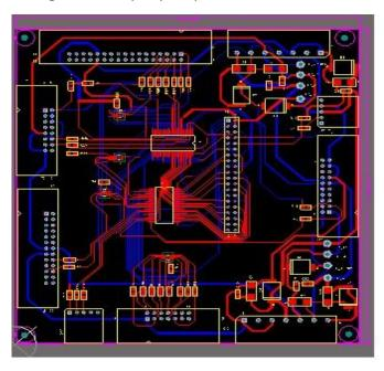
The Jig PCB for output port pins
