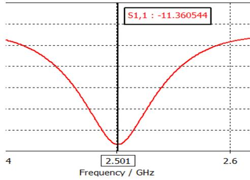
Fig 2. S11 of Aperture coupled antenna
