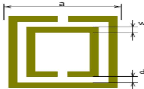
Fig 5. SRR unit cell structure
