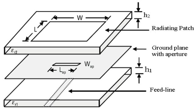
Fig 1. Aperture coupled micro strip antenna
