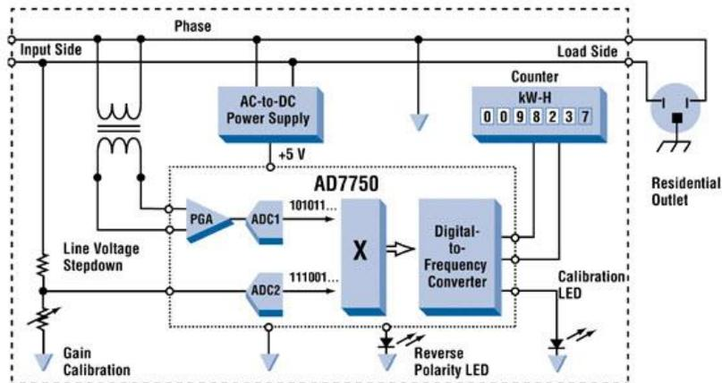
Fig:4 Analog Electronic Energy Meters
