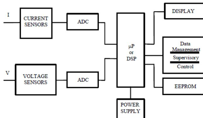
Fig: 2 Basic Scheme of digital sampling based energy meter
