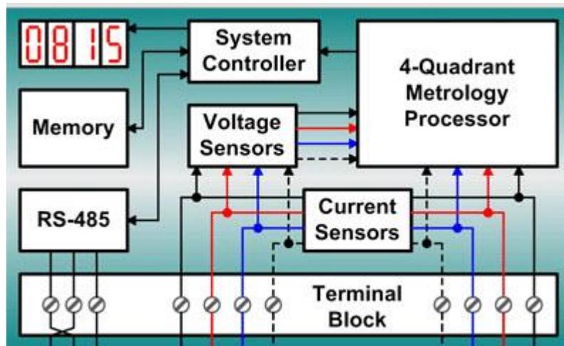
Fig: 5 Digital Electronic Energy Meters
