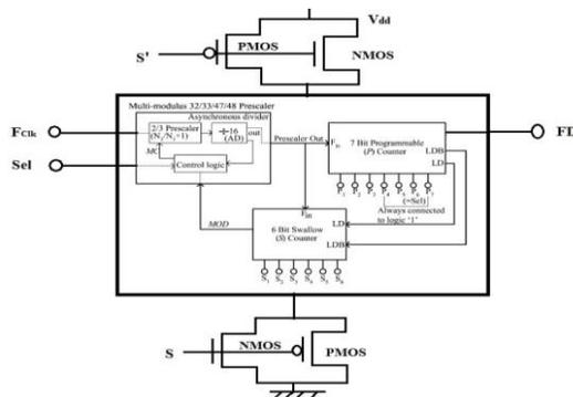
**Figure.2. Proposed dynamic logic multiband flexible divider using sleep transistor**
