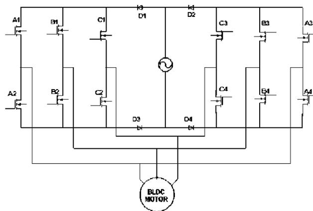
**Fig.3. Proposed Matrix Converter based BLDC motor Drive**
