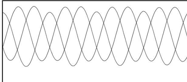
**Fig 5. Voltage Unbalance**
