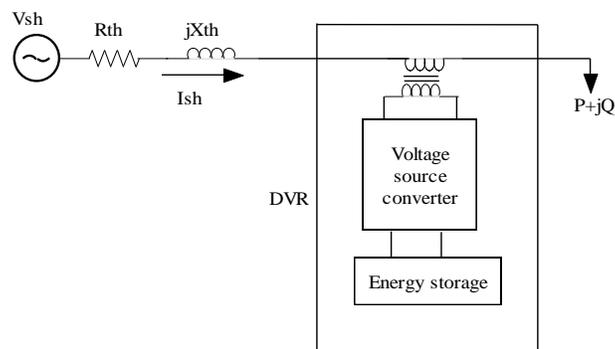
Fig 9. Block Diagram of DVR
