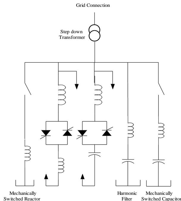
Fig 10. Block Diagram of SVC
