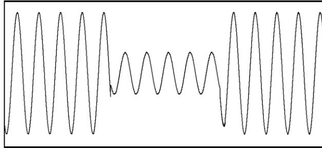
**Fig 2. Voltage Sag/Dip**
