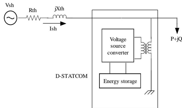
Fig 11. Block Diagram of STATCOM
