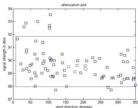
**Fig 4: received signal strength v/s wind direction in degrees.**
