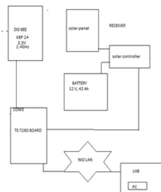
Figure 2: Internal block organization of setup
