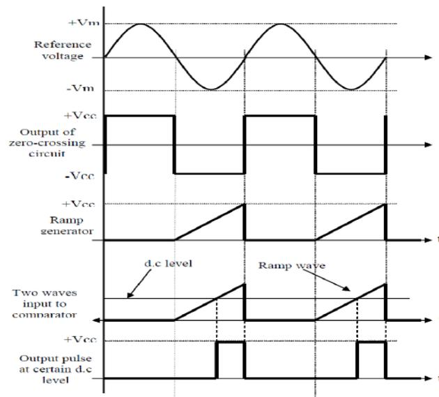
**Figure 3 The generation of gating signals of single pulse width modulation**
