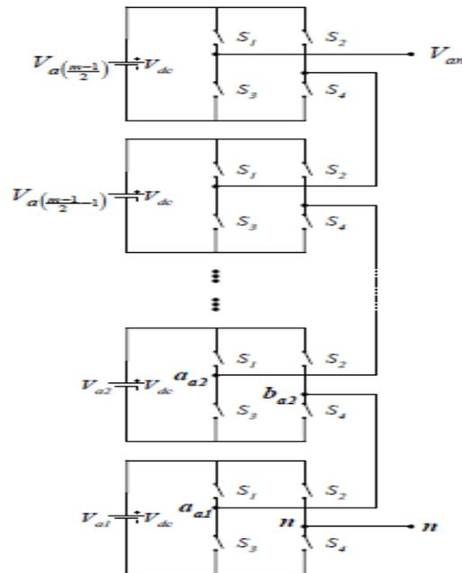
Figure 2 Cascade H bridge m level multilevel inverter
