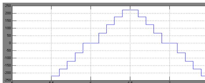
Figure 6 Simulated output voltage waveform of a multilevel inverter
