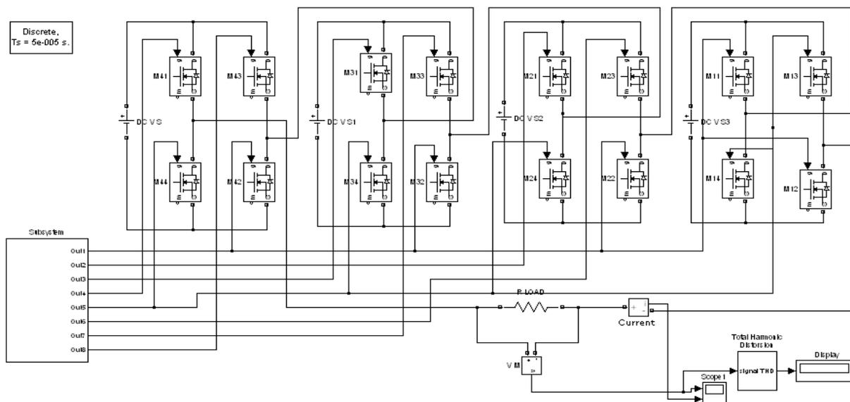
Figure 4 Simulink model for nine-level cascaded multilevel inverter
