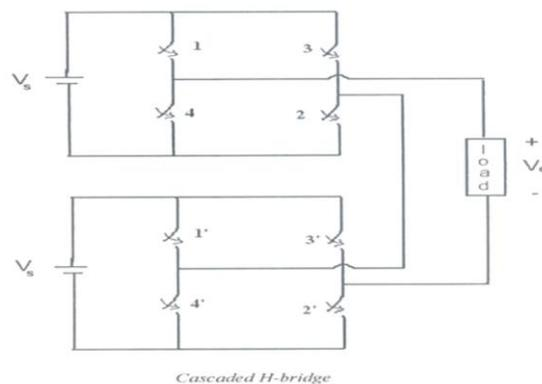
**Figure 1 Multilevel inverter topology (cascade H bridge)**
