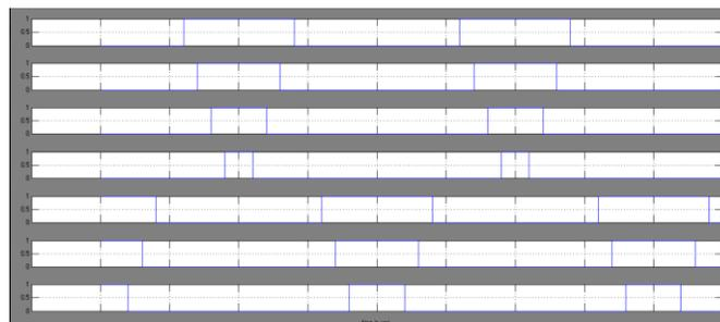
Figure 5 Gating pulses for various switches in single PWM
