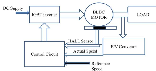
Fig 1. General figure of the motor drive system [2]
