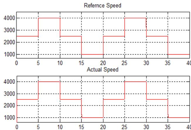
**Fig.5 Fuzzy logic controller-based BLDC drive for the given change in speed.**
