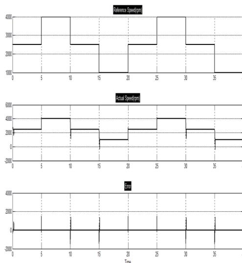
Fig.2 PI controller-based BLDC system for the given change in reference speed.
