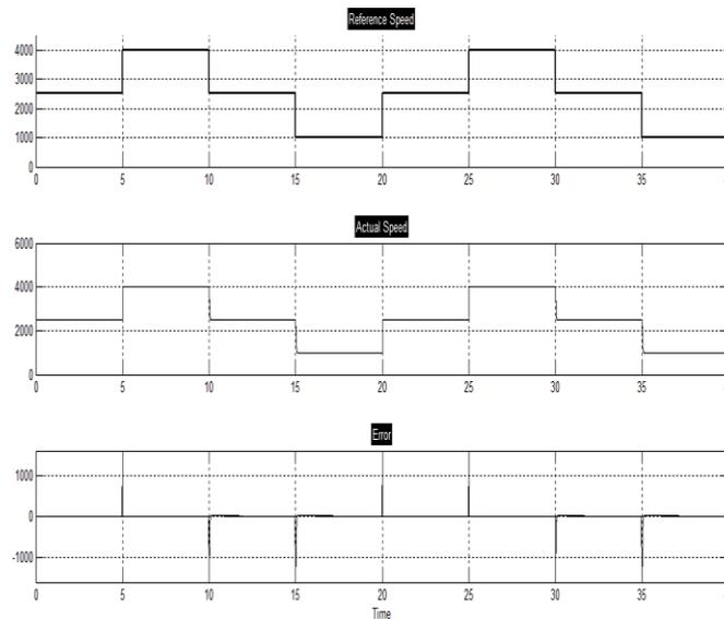
**Fig.3 PID controller-based BLDC drive system for the given change in reference speed.**
