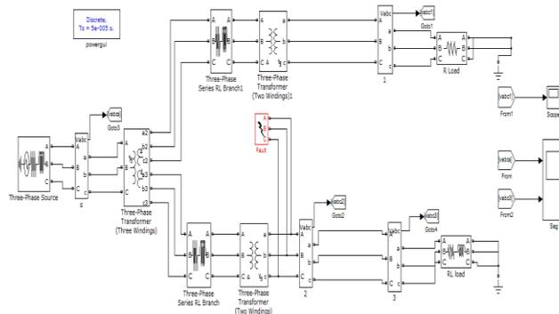
**Fig.2 Test system implemented in MATLAB to carry out the DVR simulations.**
