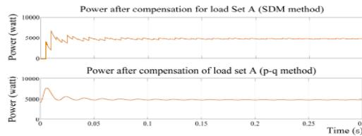
Figure 11. Overall source power after compensation for load set A
