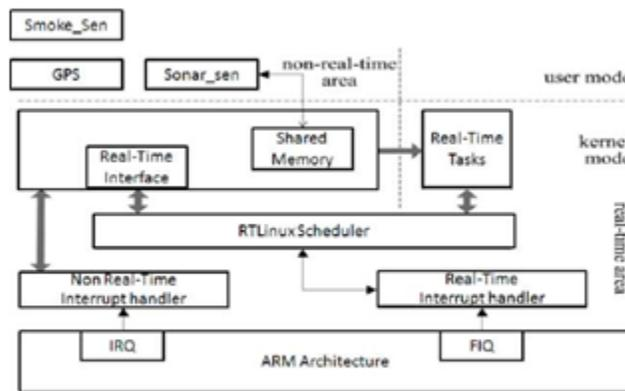
Fig. 2. Proposed Hybrid Control Architecture based on RTOS
