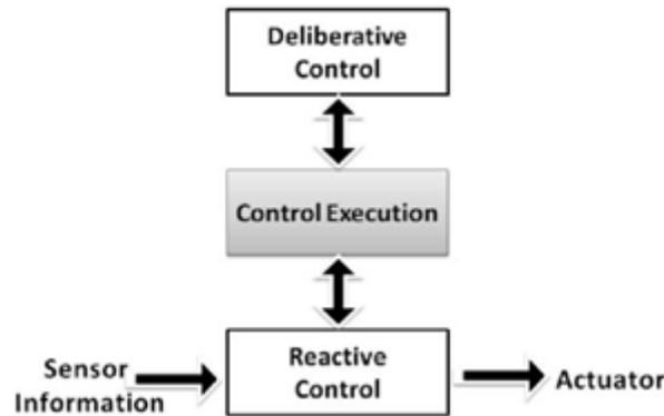
Fig. 1. Basic Hybrid Control Architecture (Perez, 2003)
