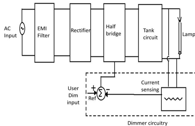
**Fig2: Block Diagram of proposed circuitry.**
