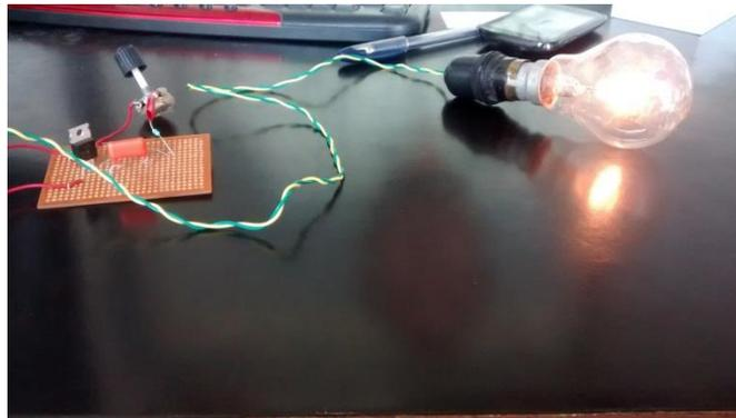
**Fig 1(b): Circuit TRIAC dimmer for incandescent lamp.**
