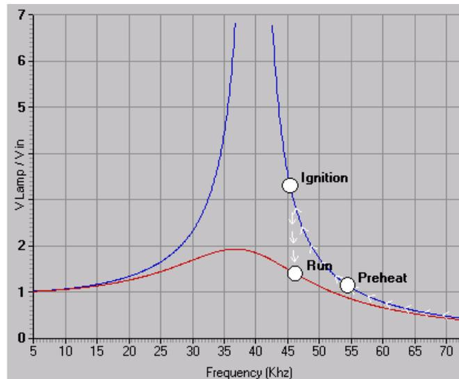
**Fig 3: Gain curve of the lamp voltage over  $V_{in}$  as a function of the switching frequency.**
