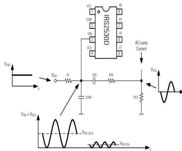
Fig 5: IRS2350D AC+DC dimming control scheme.
