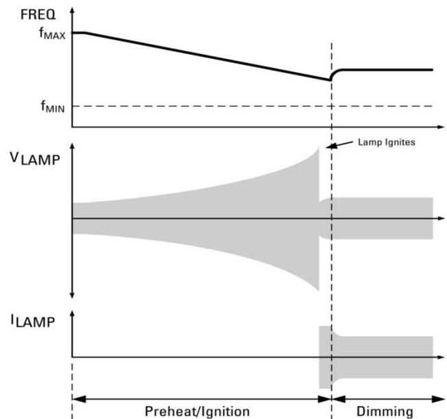
Fig 4: CFL operation timing diagram.
