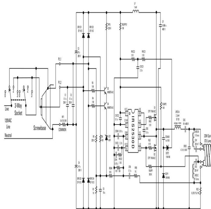
Fig 6(a): 3- way dimming circuit using IC IRS2530D.
