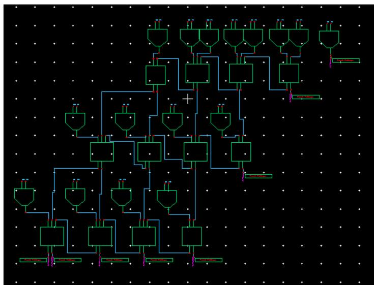
Fig 7: 4-bit Array multiplier using conventional MA
