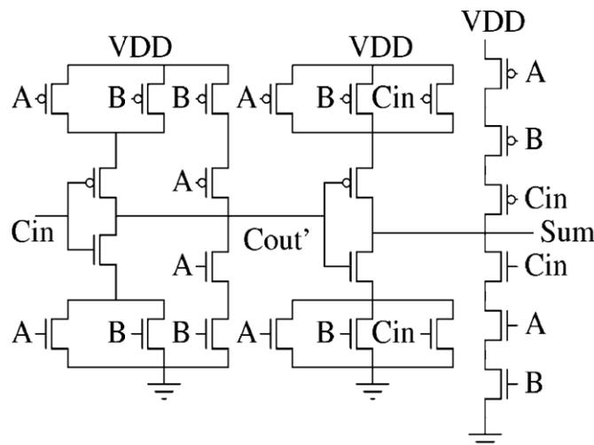
Fig 1. Conventional Mirror Adder [1]
