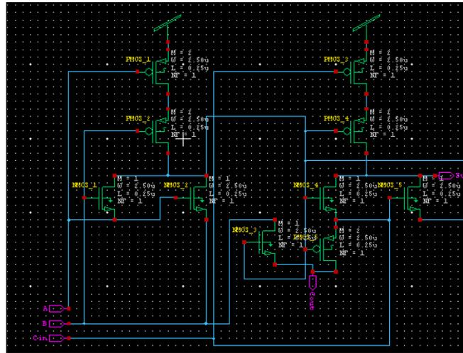
Fig 4: Schematic of adder with 10 transistors
