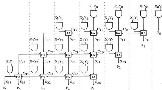
Fig 6: Design of 4-bit Array Multiplier
