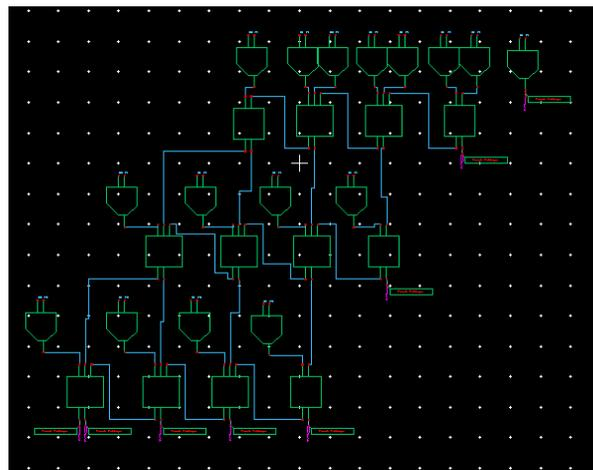
Fig 9: 4-bit Array multiplier using proposed adder
