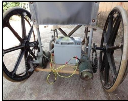
**Figure 4. Motor & Gear Arrangement**
