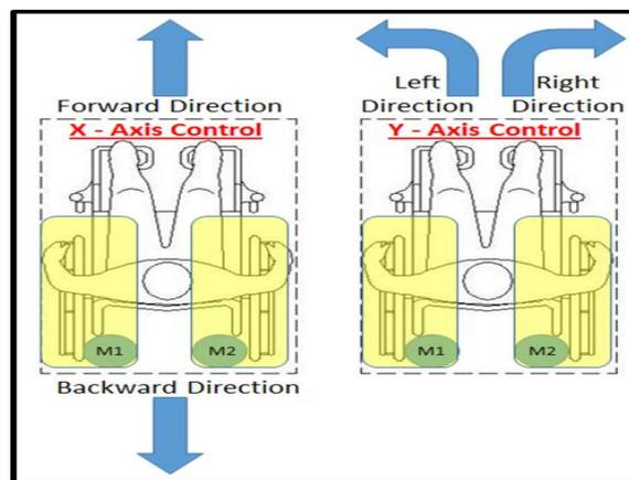
Figure 2. X-Axis and Y-Axis Control of accelerometer
