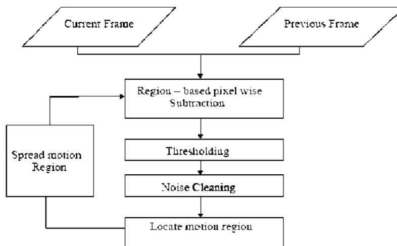
Fig 3.2 Block Diagram showing Object Tracking Algorithm
