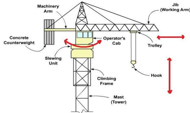
**Fig.2d: A tower crane's degree of freedom.[17]**
