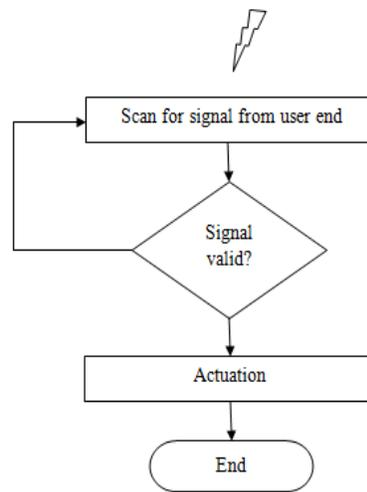
**Fig.3b: Flowchart of the system (Remote end)**
