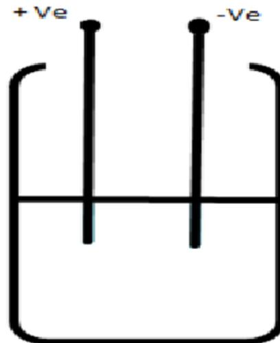
Fig. 4 urine level detector
