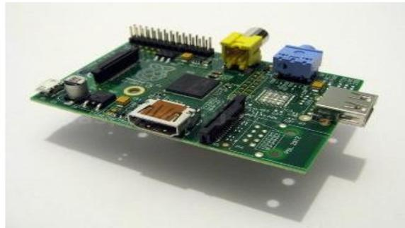
**Fig.3: Raspberry pi board**
