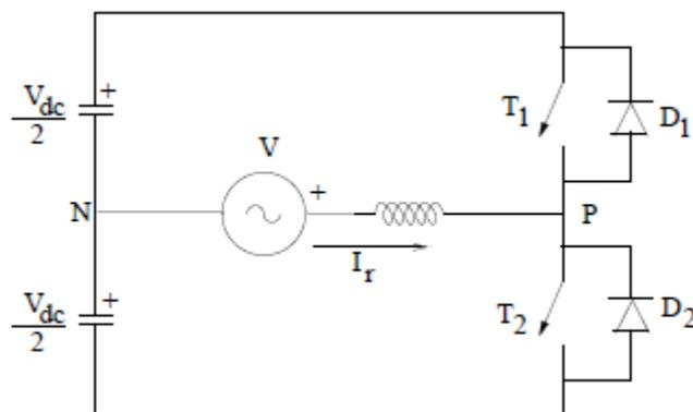
Fig. 1 A single phase StatCom
