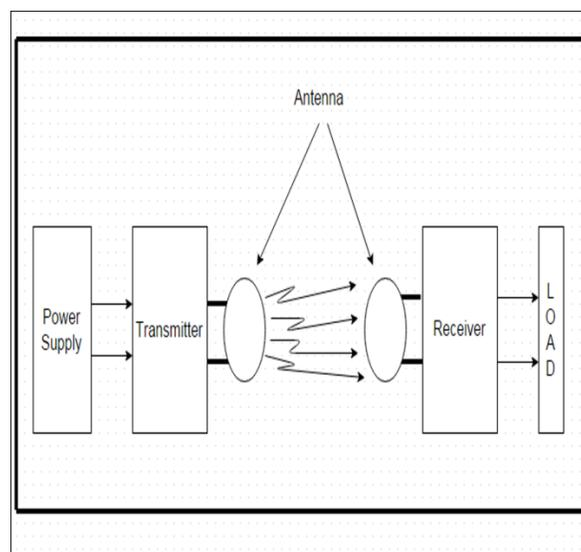
In general a wireless power system consists of a "transmitter" device connected to a source of power such as mains power lines, which converts the power to a time-varying electromagnetic field, and one or more "receiver" devices which receive the power and convert it back to DC or
