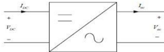
**Figure 1: General Block Diagram of Inverter**
