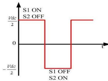
Figure 3.1.2: Inverter Output
