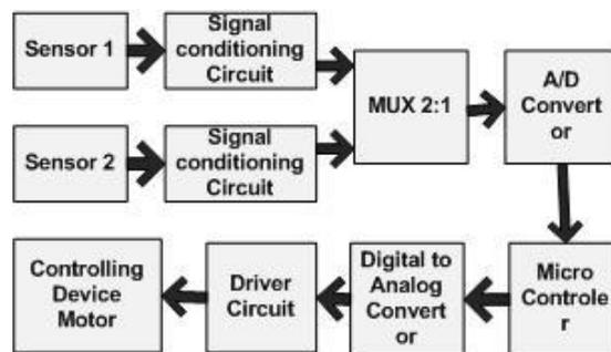
**Figure 2. Intelligent control system of ASO-Ankle foot**
