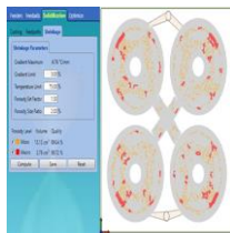
Fig. 09 Shrinkage in old design
