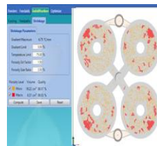
Fig. 09 Shrinkage in improved design
