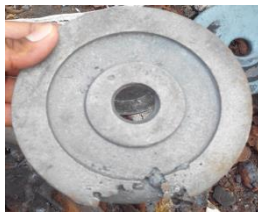
Fig2.defect in circular disc casting Fig 3 . 3D CAD and simulation result of disc without feeder system
