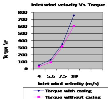
Graph of inlet wind speed Vs. Torque
