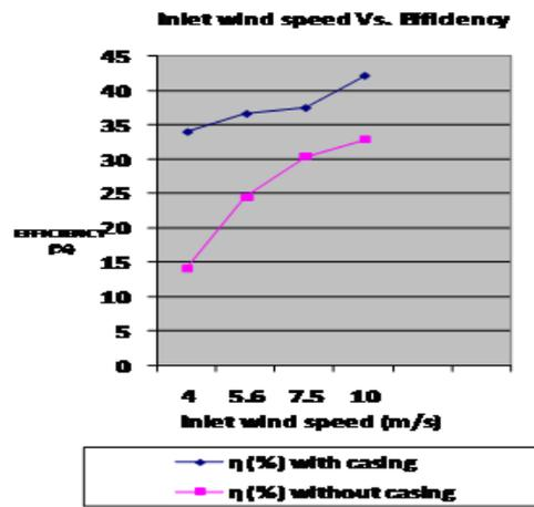
Graph of inlet wind speed Vs. Efficiency
