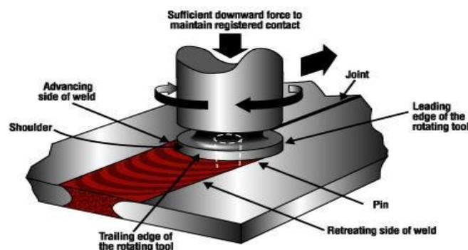
Figure No.1.1 Friction stir welding
