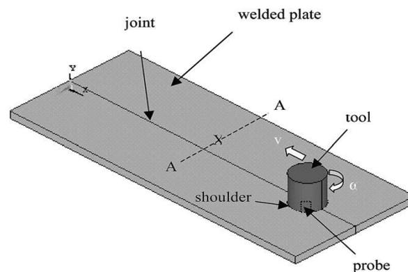
**Figure No.2.1 A schematic representation of the Friction stir welding process**
