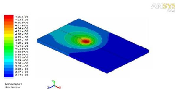
Figure No.4.1.HDPE sheet Temperature distribution in Ansys
