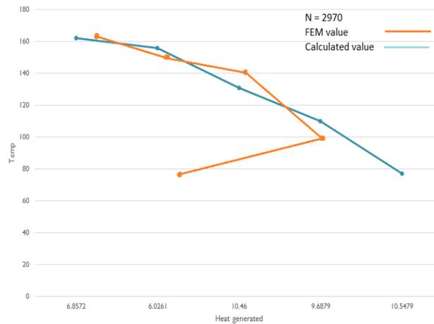
**Graph No.4.2 - A comparison of calculated and measured Temperature with Heat generated**
