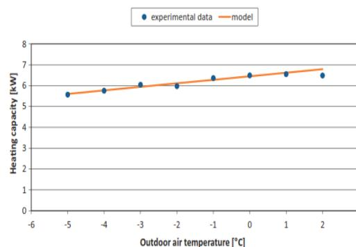
**Fig.1 Heating capacity as a function of outdoor air temperature [6].**
