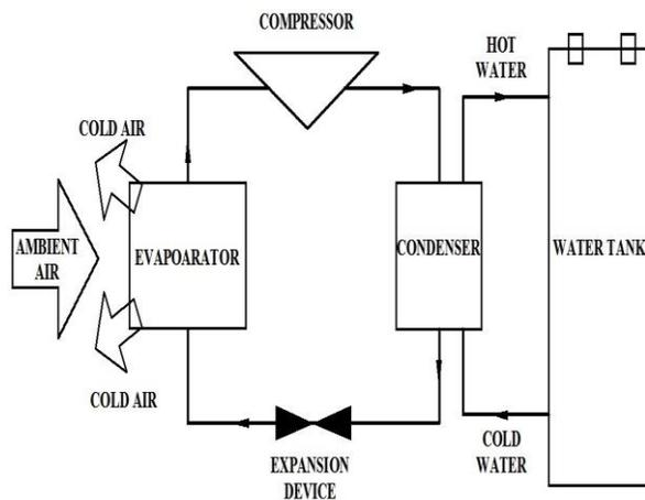
Fig.1 Schematic of a simplified heat pump water heater system [5]
