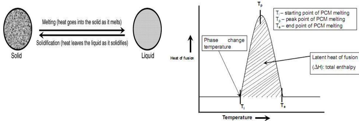
Fig.2.1. Schematic representation of phase change process [2]
