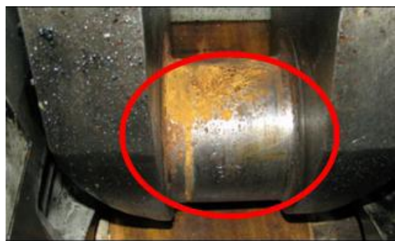
Fig.6.1 Damage to journal surface of hardening
