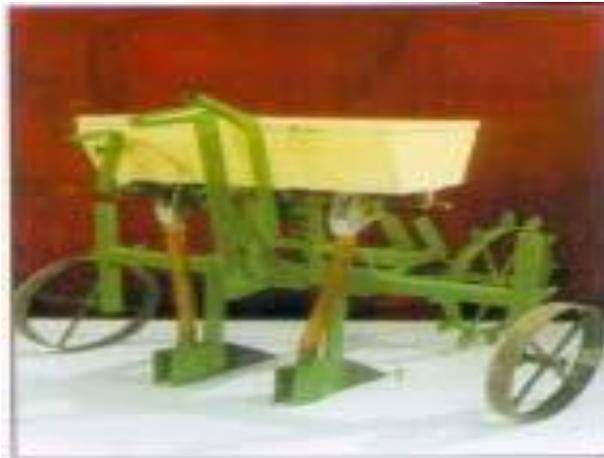
4. TWO ROW SEED CUM FERTILIZER DRILL: It is an animal drawn simple, light weight and compact machine to sow crops like wheat, gram, sorghum, soybean, lentil, pea, sunflower, safflower etc and drill fertilizer in black soil under rained condition. The fluted roller metering mechanism, fitted in the unit, gets the drive from ground drive wheel of 300mm diameter through chain and sprocket. The shoe type furrow opener with non-clogging boot place the seed at desired depth.
