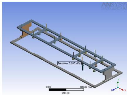
Figure No 5.6: Force acting on top clamp.
