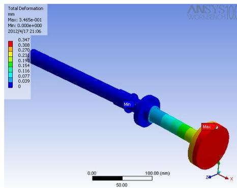
Figure No 5.3: Deformation of shaft.
