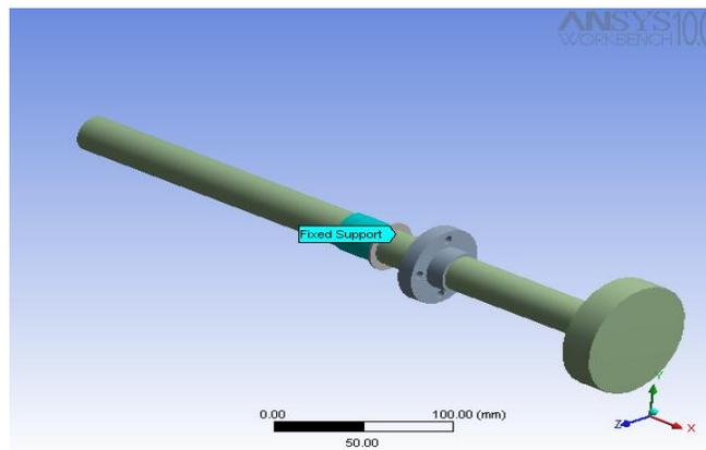
Figure No 5.1: Fixed support acting on shaft
