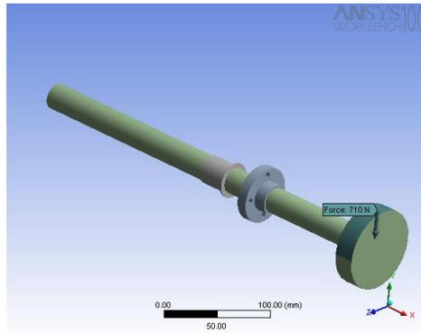
Figure No 5.2: Force acting on shaft.
