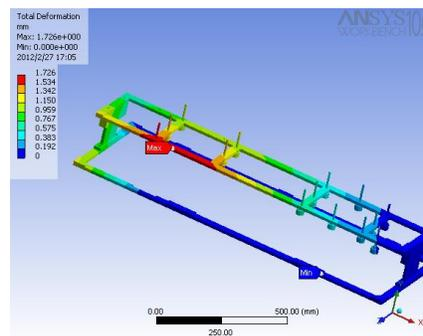
Figure No 5.7: Deformation of top clamp assembly.
