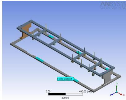
Figure No 5.5: Fixed support acting on top clamp.
