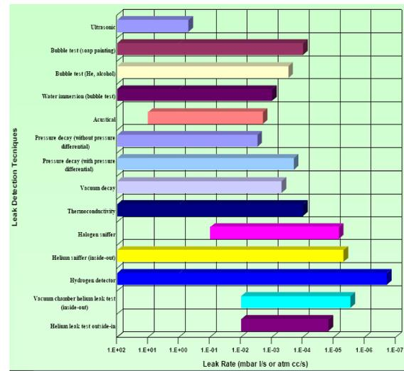
Figure No. 3.1- Various Leak Detection Techniques vs. Leak Rate.
