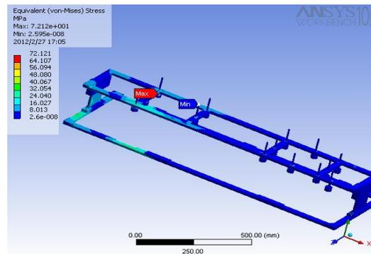
Figure No 5.8: Stresses on top clamp assembly.
