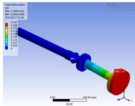
Figure No 5.4: Deformation of shaft
