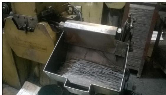
Figure 4.3: Cut wire collected in container
