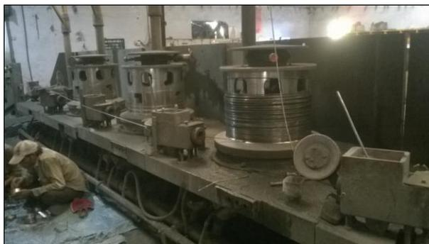
Figure 4.1: Wire Drawing Process
