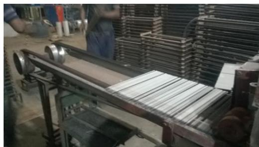
**Figure 4.7: Finishing of electrodes**
