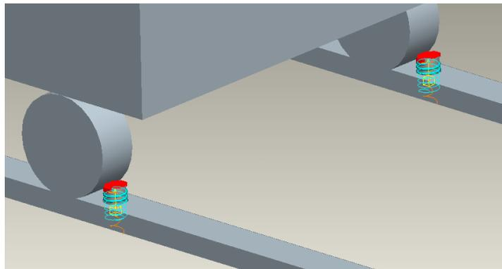
Figure 5.4: Spring stopper having weight sensor
