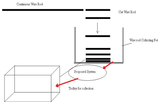
Figure 5.1: Conceptual model of system
