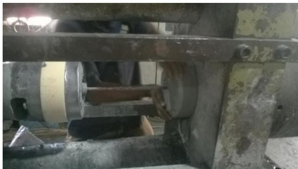
**Figure 4.5: Flux coating by extrusion**
