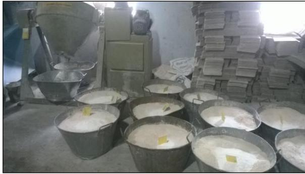
**Figure 4.4: Powder formed for flux coat preparation**
