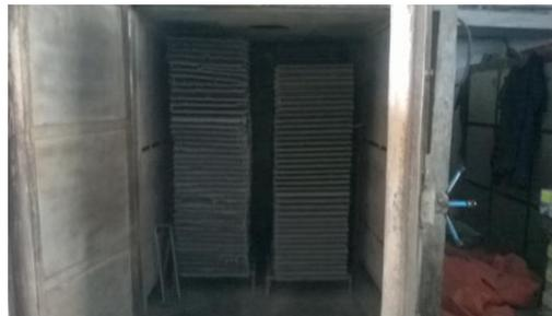
**Figure 4.6: Flux de-moisturizing in oven**
