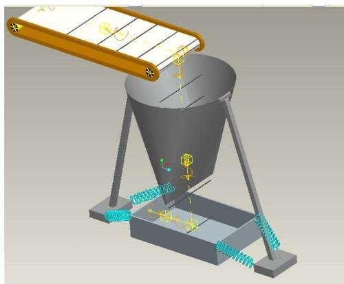
Figure 5.2: Electrode collecting hopper (Design I)
