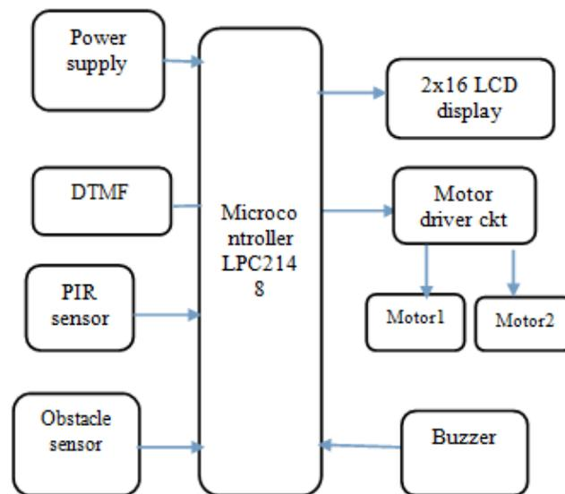
**Figure 5: Block diagram of proposed system**
