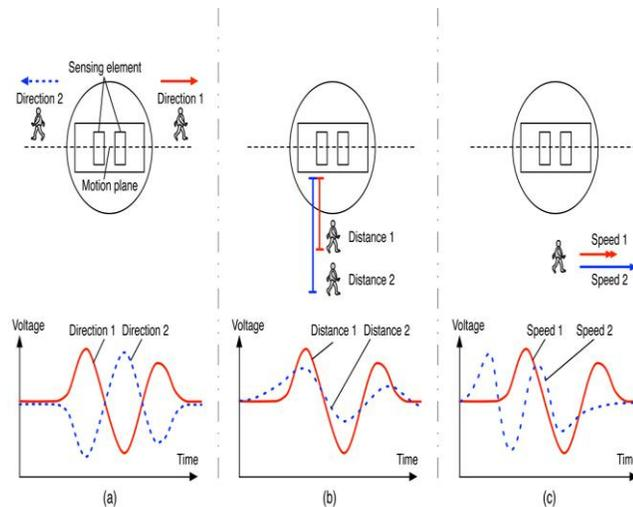
The changes in the amount of infrared striking the element change the voltages generated, which are measured by an on-board amplifier.
