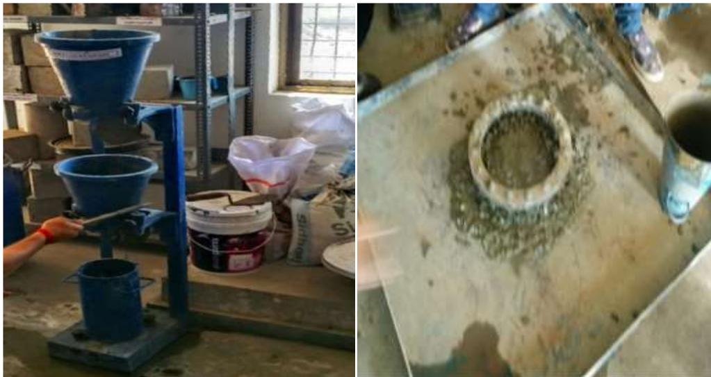
Fig – 1 (a) Compaction Factor Test
