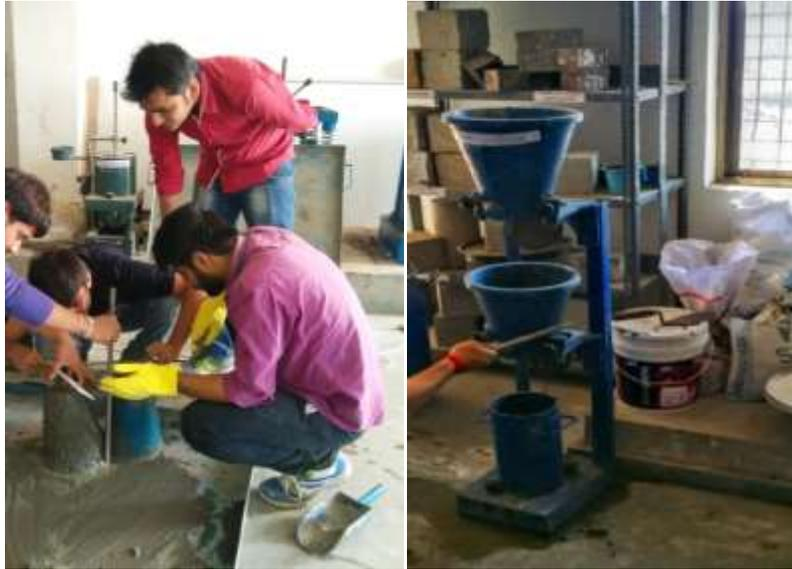
Fig – 1 (a) Slump Test
